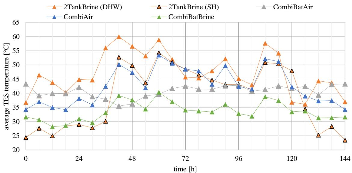
Figure 8: Average temperature of the TES-tanks during the 6-day system test.
