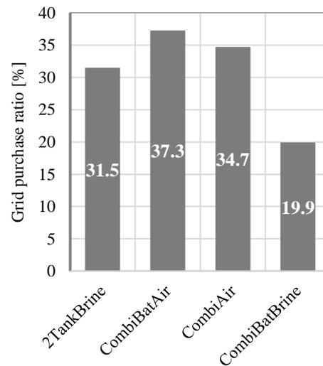
Figure 7: Grid purchase ratio of the tested systems.
