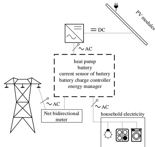
Figure 2: Fixed (galvanically integrated) measuring points. In addition, non-contact measurements are carried out within the tested system.
