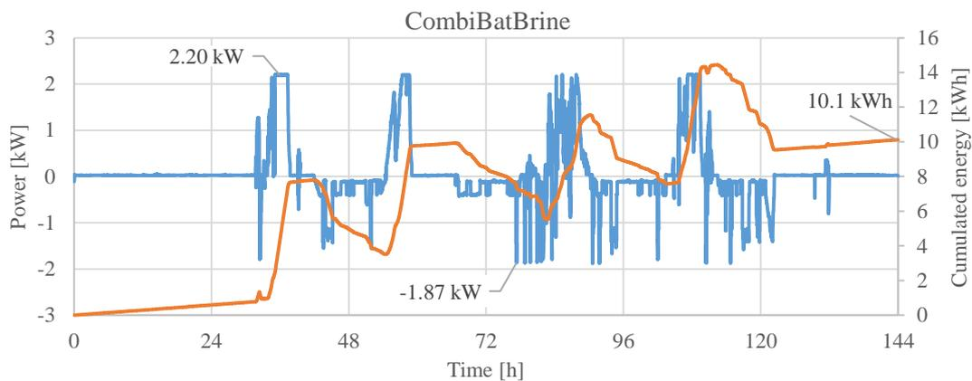
Figure 11: Electrical power of the charging and discharging of the battery as well as the cumulative energy during the 6-day test.
