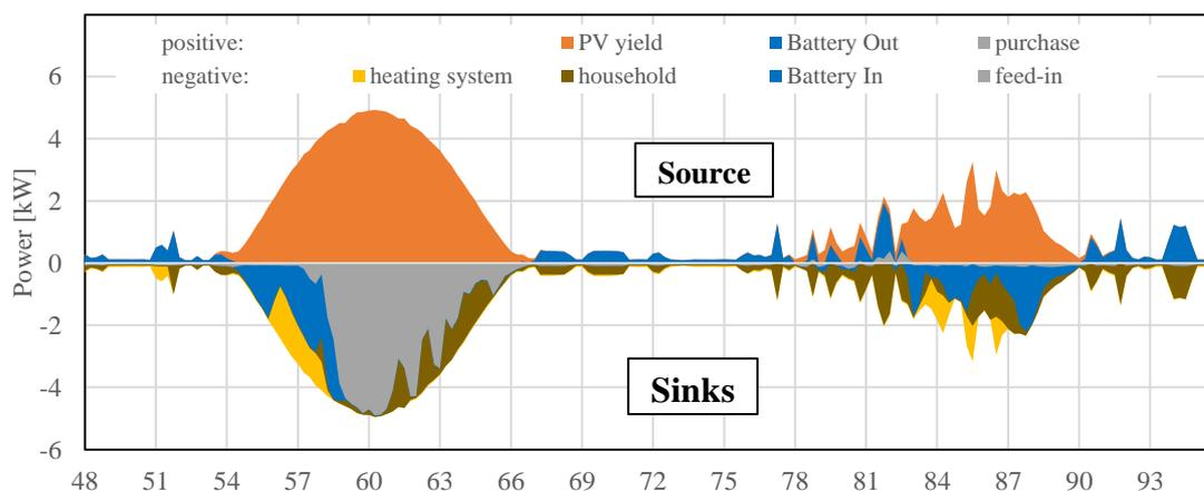
Figure 9: Excerpt of the measurement of System CombiBatBrine: Measurement of electric power during the days 3 and 4 of the 6-day test sequence.
