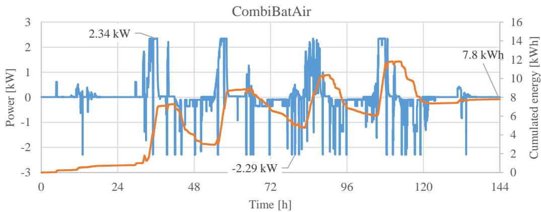
Figure 10: Electrical power of the charging and discharging of the battery as well as the cumulative energy during the 6-day test.
