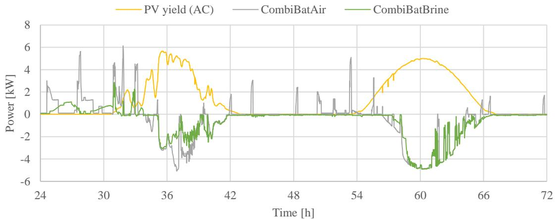
**Figure 12:** Excerpt of two system tests: PV yield (yellow) and the grid purchase (positive values green or grey) and feed-in (negative values) during a period of two days within the 6-day test.
