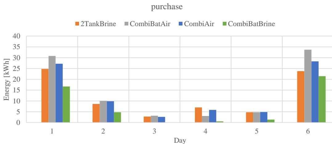
Figure 5: Electric energy from the grid per day.
