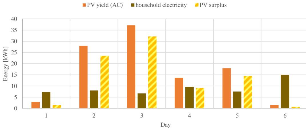
Figure 3: PV yield and household electricity and PV surplus per day. The calculation of PV surplus is based on minutes.
