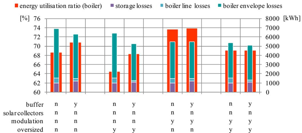
**Figure 4: Influence of the integration of the pellet boiler on the degree of utilization of the boiler and the heat losses through pipes, TES and boiler. The results of annual simulations are presented by pairs that differ in the integration of the pellet boiler to the buffer store or via a low loss header directly to the space heating circuit. Source: Konersmann et al. 2011.**
