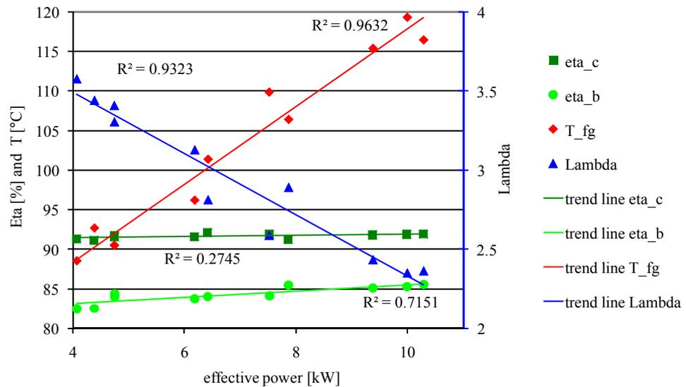
**Figure 1: Measurement results of an pellet boiler in steady state operation in different modulation stages, based on the net heating value. Combustion efficiency (eta\_c), boiler efficiency (eta\_b), flue gas temperature (T\_fg) and excess air (Lambda). Source: Konersmann et al. 2007.**
