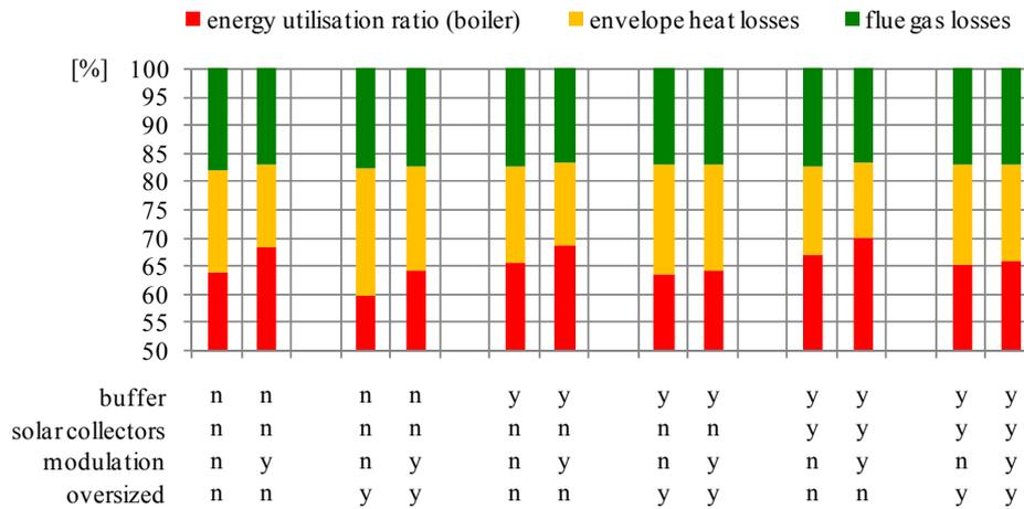
**Figure 2: Results of system simulations with a pellet boiler that was implemented in different heating systems. Results based on the gross heating value. The results are arranged in pairs that differ in the modulation capability. Source: Konersmann et al. 2011**
