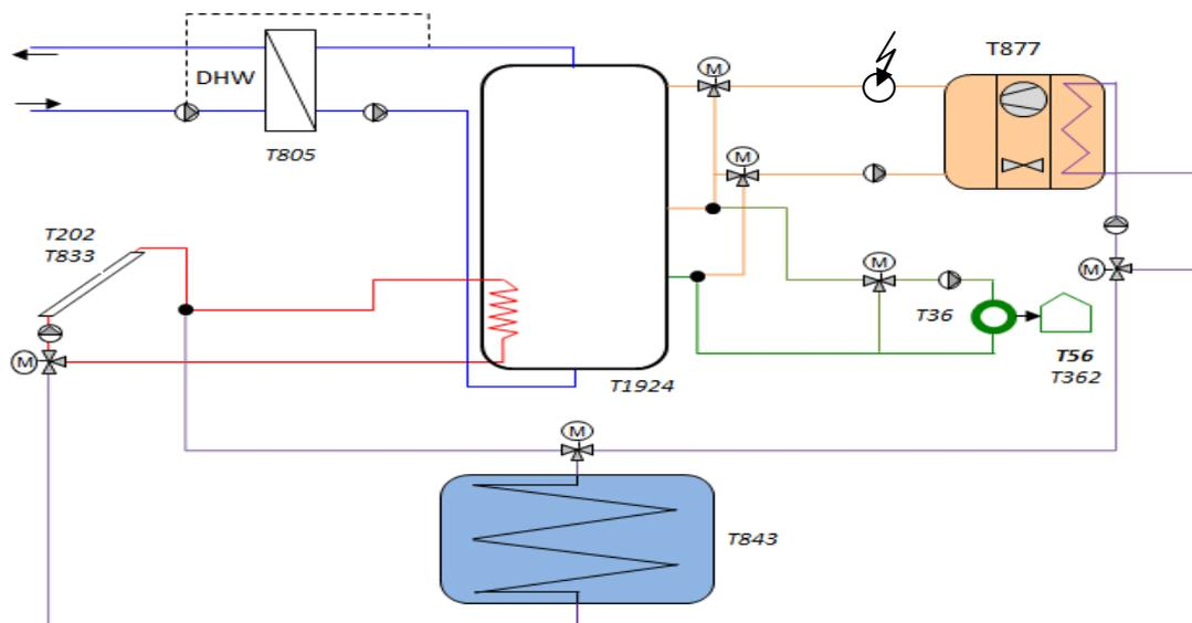
Figure 2: Hydraulic schema of the both alternative systems;  $T_{xy} = \text{TRNSYS Type number } xy$
