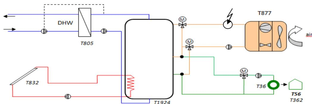
Figure 1: Hydraulic scheme of the reference system;  $T_{xy} = \text{TRNSYS Type number } xy$
