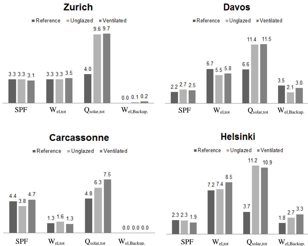
Figure 4: Result summary of the comparison of all three systems, all energies in MWh
