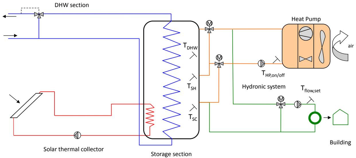
**Figure 2:** Schematic of the combined thermal solar collector and air source reference system with its temperature sensors for charging the storage ( $T_{DHW}$ ,  $T_{SH}$ ,  $T_{SC}$ ) and to control the heat pump ( $T_{HP,on/off}$ ) as well as flow temperature to the heating system ( $T_{flow,set}$ ) [22]
