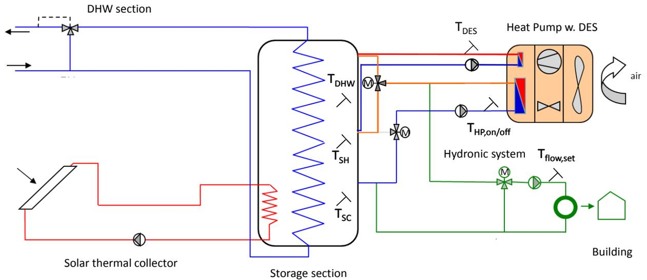
**Figure 4:** Schematic layout of adapted combined solar and heat pump system by integrating the DES in the hydrionic system according to strategy 5
