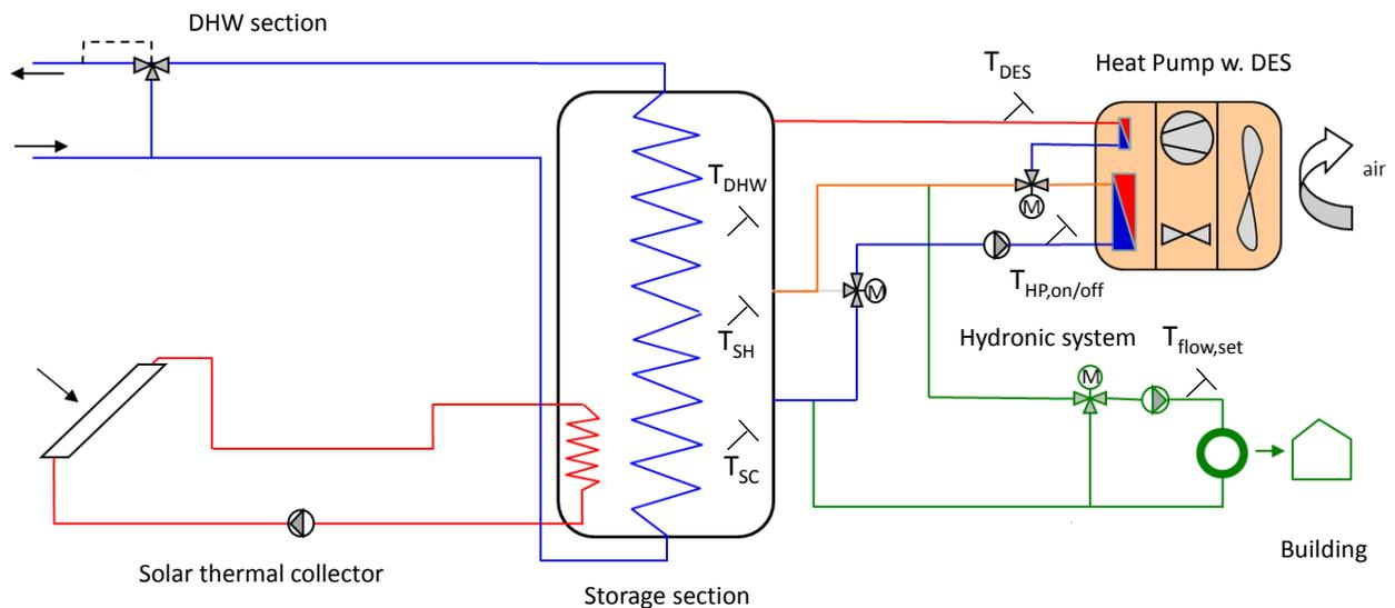
**Figure 3:** Schematic layout of adapted combined thermal solar and heat pump system by integrating the DES in the hydronic system according to strategy 1 to 4
