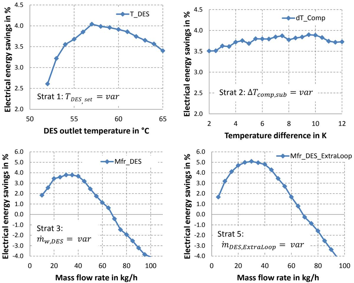
**Figure 7:** Annual system simulation results of the variation study for the strategies 1, 2, 3 and 5 by using different values for the parameters
