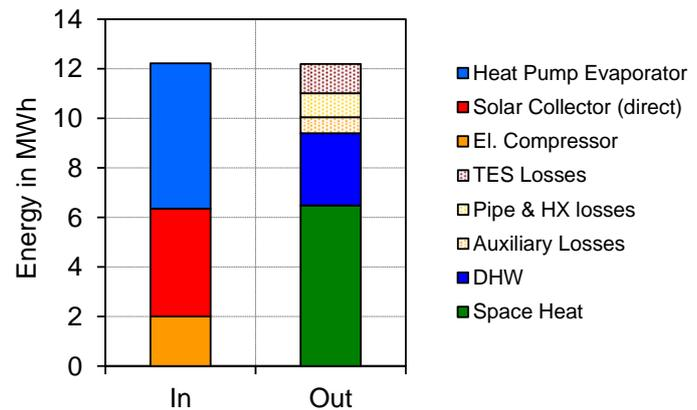
**Figure 8:** Energy balance of strategy 1 ( $t_{DES,set} = 57$  °C) with all energy inputs into the system (left) and energy outputs (right)
