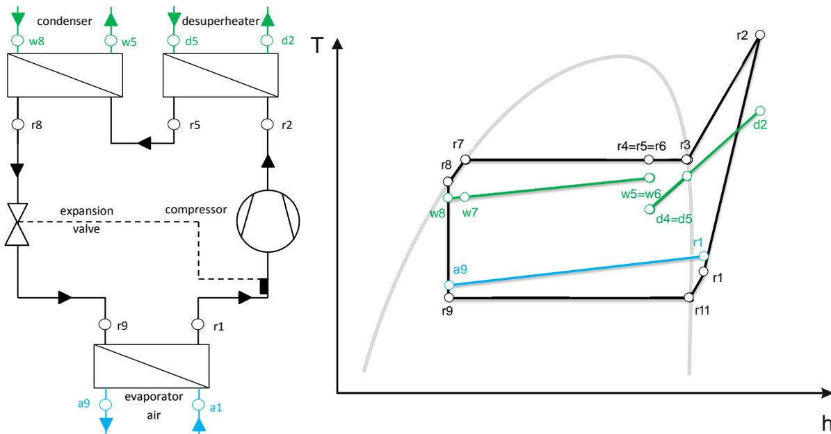
**Figure 1:** Left: Schematic layout of the heat pump cycle including the desuperheater; Right: Corresponding exemplary process in the temperature-enthalpy-diagram (T-h-diagram) with all heat exchangers active [19]
