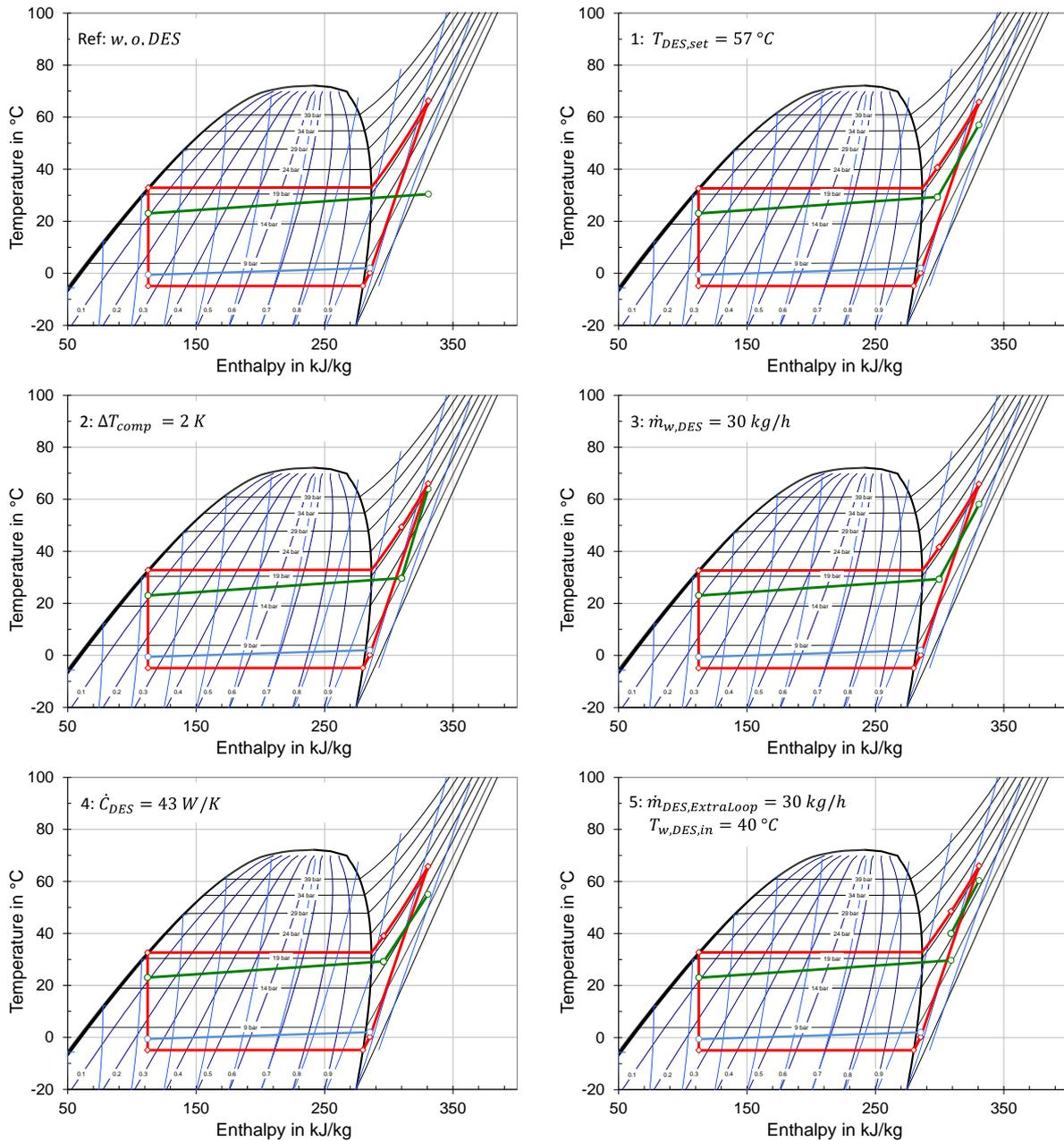
**Figure 5:** Steady state results of reference system (Ref) and strategy 1 to 5 at exemplary operating conditions (A2W30) in a temperature-enthalpy diagram for R410A
