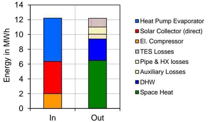
**Figure 6:** Energy balance for the reference system with all energy inputs into the system (left) and energy outputs (right)
