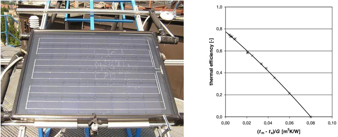
Fig. 1. (a) Glazed PVT collector with siloxane gel lamination; (b) thermal performance characteristic from experimental tests.
