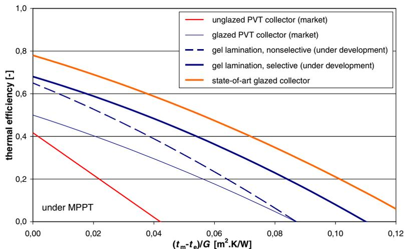
Fig. 2. Thermal efficiency characteristics of PVT collectors used for performance modeling in the analyses.
