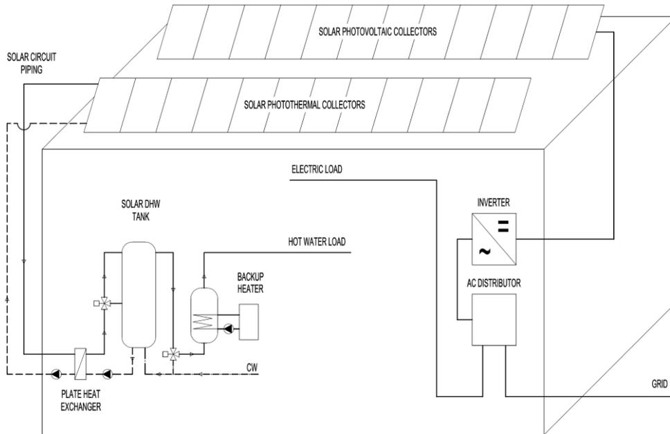
Fig. 3. Simplified scheme of the considered solar energy system for block of flats.
