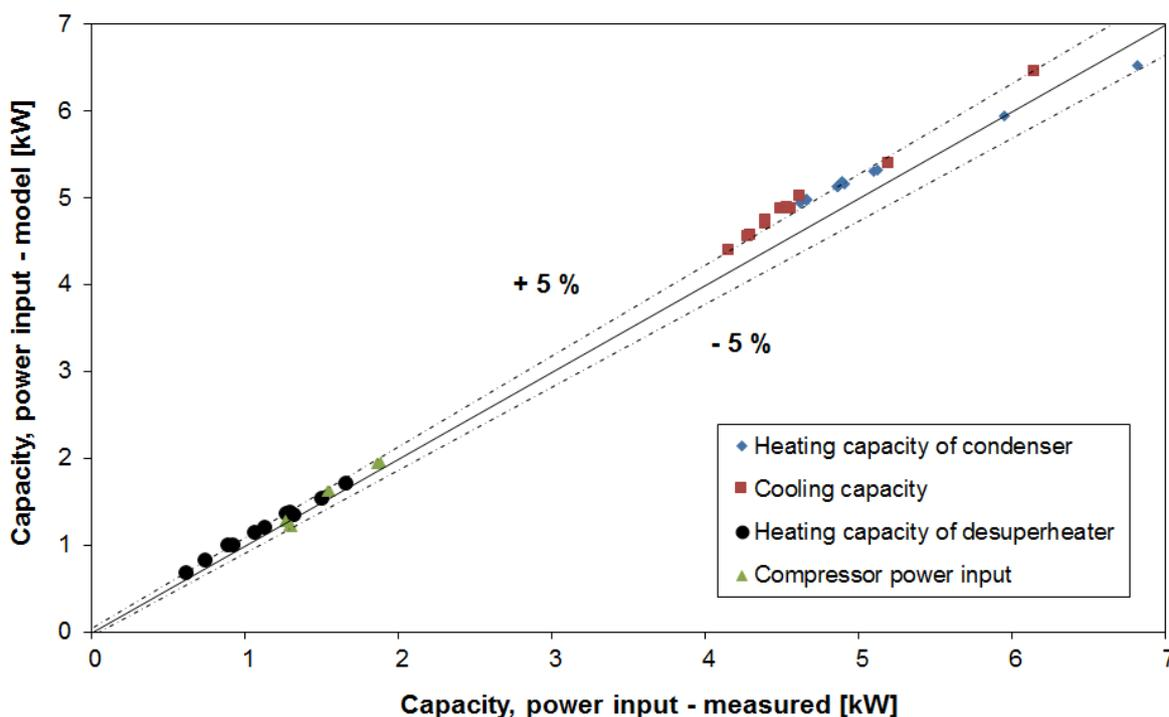
Figure 10: Verification in condenser/desuperheater mode.
