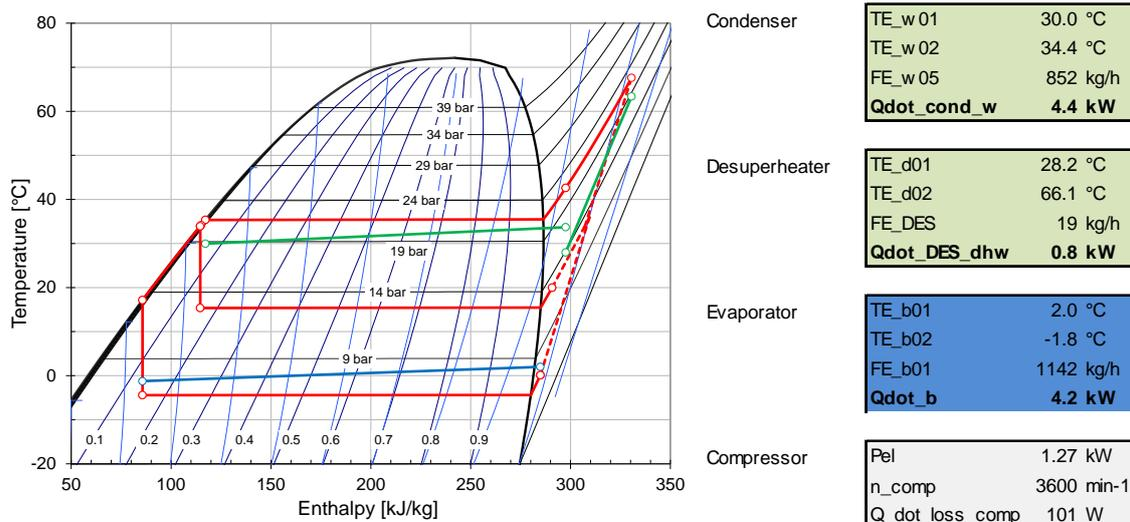
Figure 5: Measured result (example) of the final heat pump prototype in a temperature-enthalpy-diagram.
