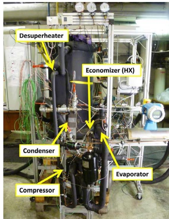
Figure 4: Photo of the final heat pump prototype.
