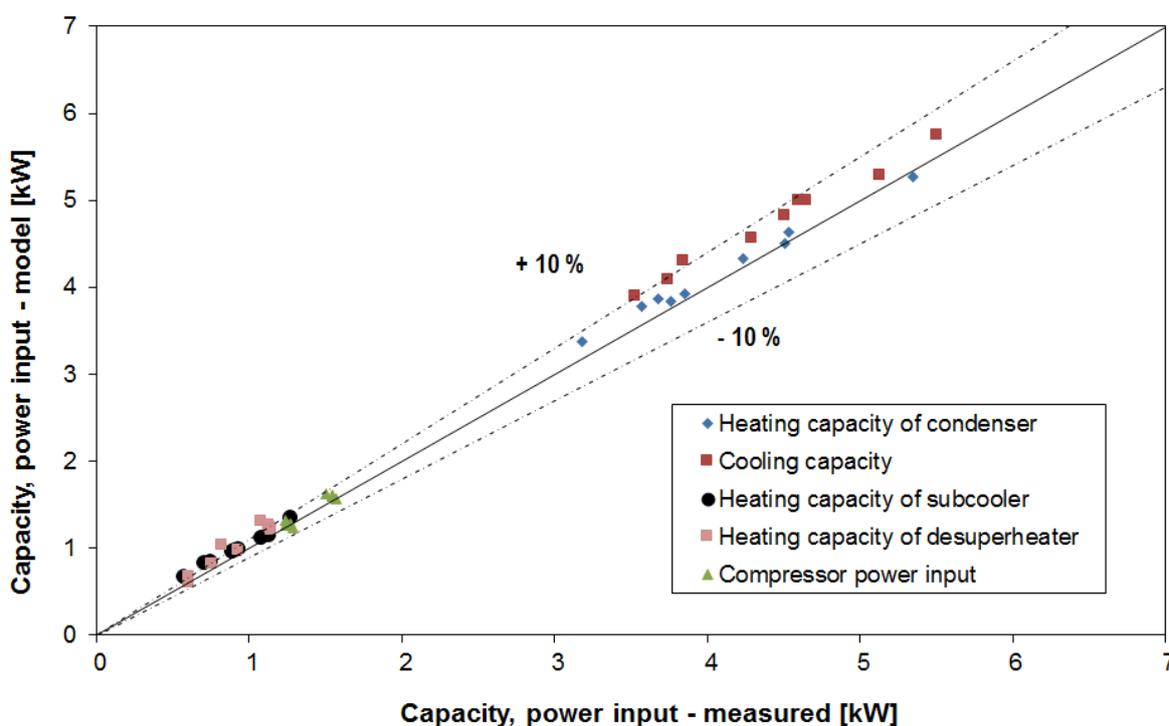
Figure 11: Verification in triple sink mode
