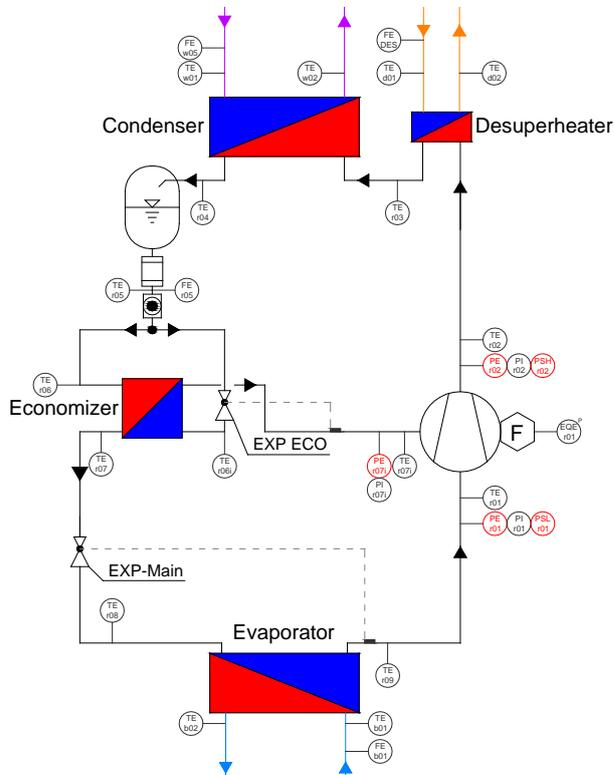
Figure 3: Scheme of the heat pump prototype with its measurement equipment.
