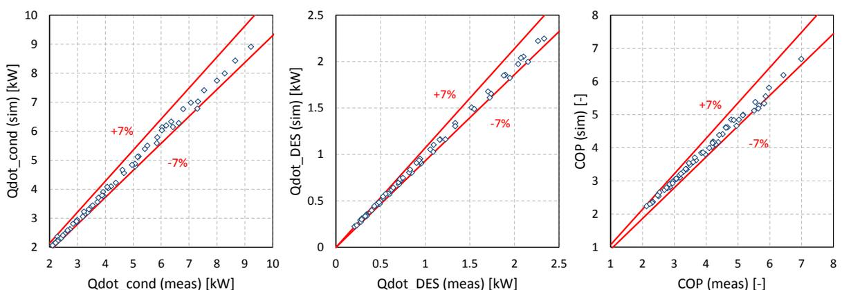
Figure 6: Simulation results from the heat pump model vs. experimental data from the heat pump test rig (58 measurement points).
