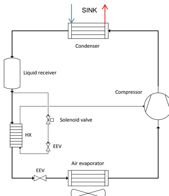
Figure 7: Scheme of the heat pump prototype.
