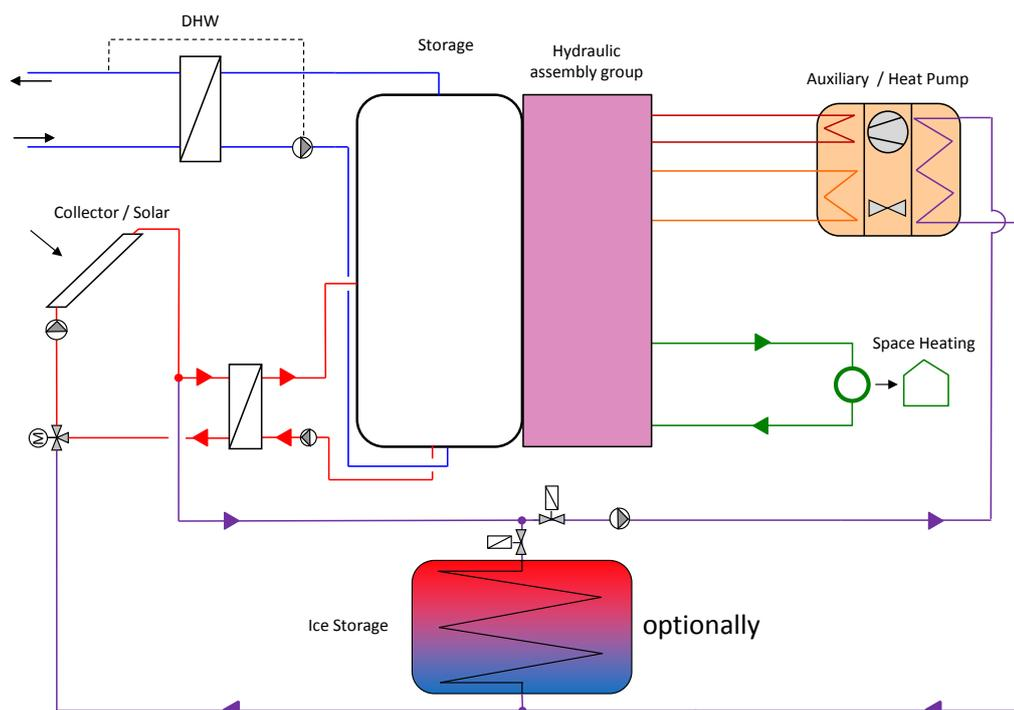
Figure 2: Schematic of the optimized system developed by ESSA, IWT and SPF.
