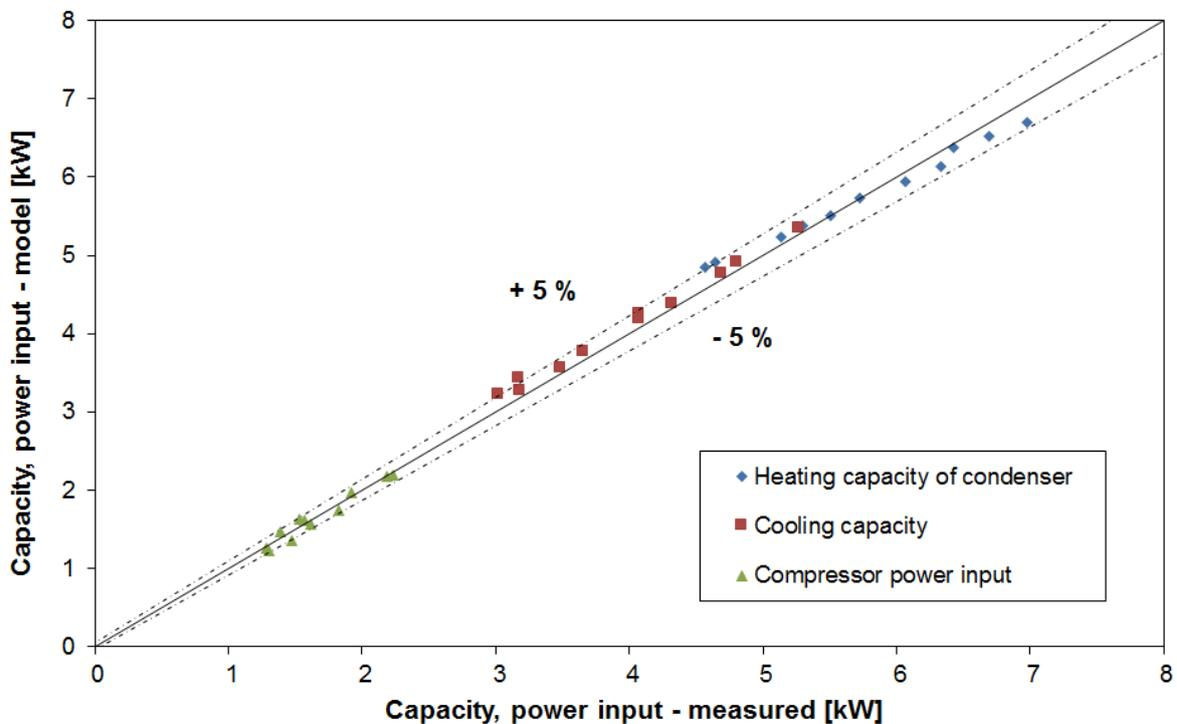
Figure 9: Verification in condenser mode only.
