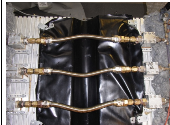
Figure 5: (after test) Corrugated pipe taken out of insulating tube.
