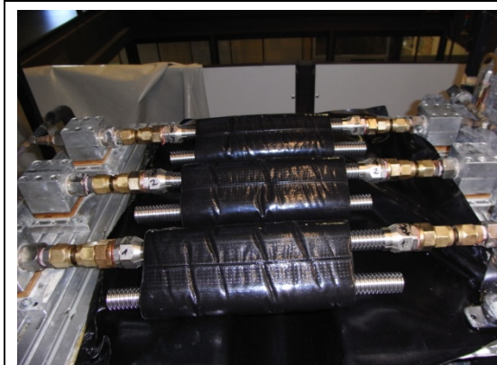
Figure 3: (before test start) Detail of installed test samples before testing. For each sample one of the tubes was connected and tested. The second tube is not considered.
