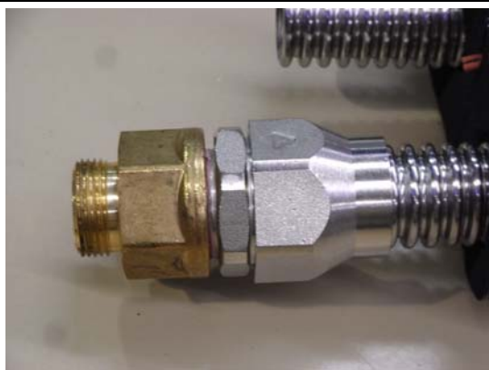
Figure 2: (before test) Compression fitting.
