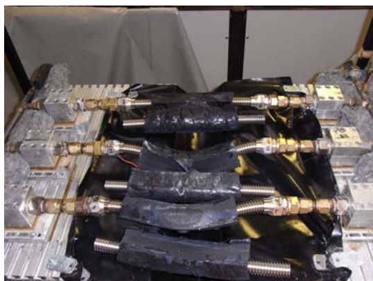
Figure 4: (after test) No leakage was observed. The EPDM insulation of the two tubes was separated and the UV-protection foil was overheated. This is due to the harsh condition during the test. In a normal installation the thermal load on the insulation is much smaller.
