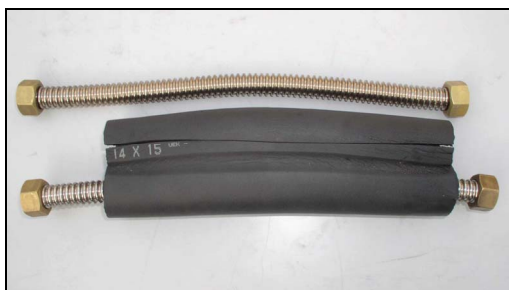
Figure 5: (after test) Corrugated pipe taken out of insulating tube.
