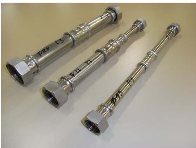
Figure 6: (after test) All the samples are fully intact and no leakage has been observed during the whole test procedure.
