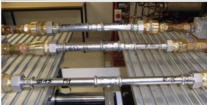
Figure 5: (before test start) Test samples installed on the test rig.
