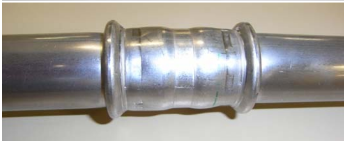
Figure 4: (before test start) Test sample 3, 6222808 – pipe 1.4521 Ø28
