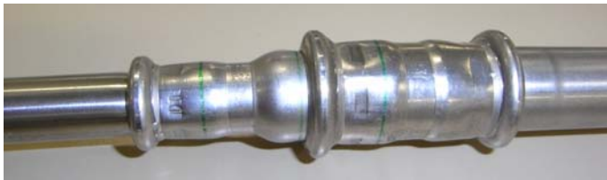
Figure 3: (before test start) Test sample 2, 611791.4 – pipe 1.4404 Ø15
