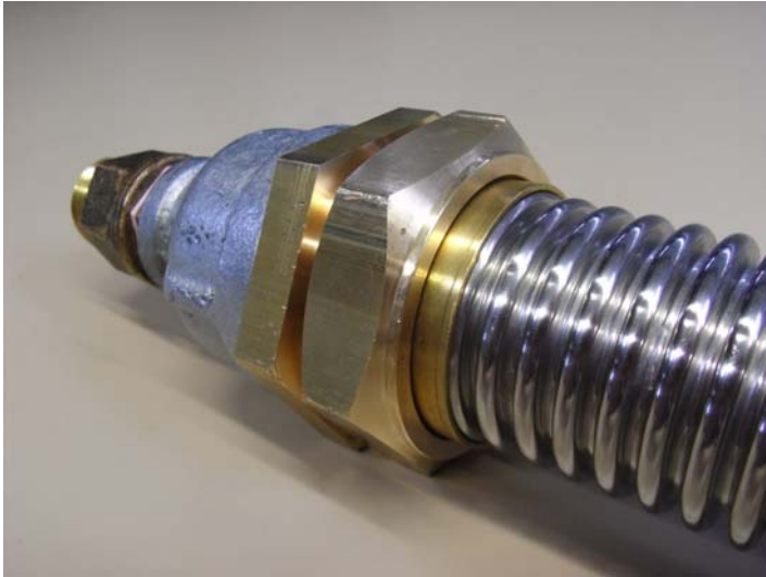
Figure 3: (before test start) Close view on ready installed coupling system.
