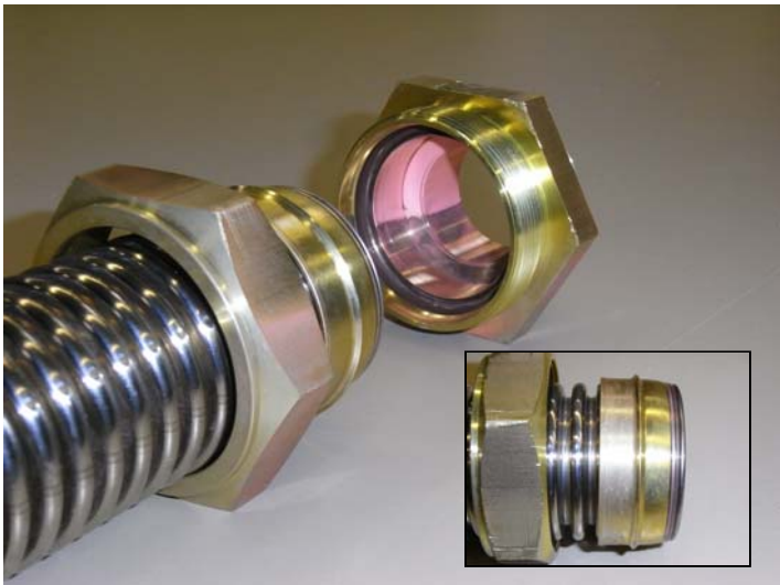
Figure 7: (after test) Close look at the opened test sample. No visible signs of deterioration that could indicate reduced lifetime or leakage.
