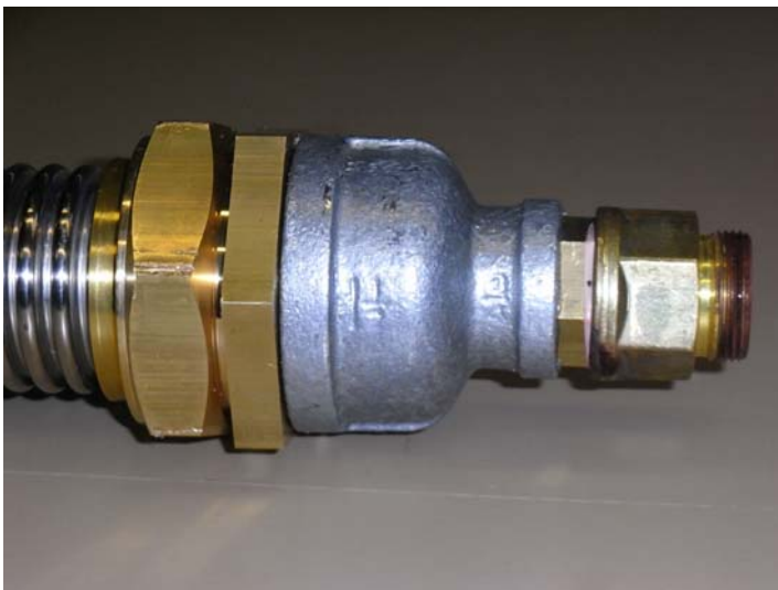
Figure 4: (before test start) The grey cast metal adapter is not part of the test and is needed to connect the samples to the test bench.
