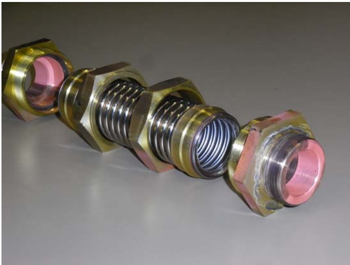
Figure 6: (after test) Opened test sample. No visible signs of deterioration that could indicate reduced lifetime or leakage. The red colour inside the connectors is a sign of overheating during the test.
