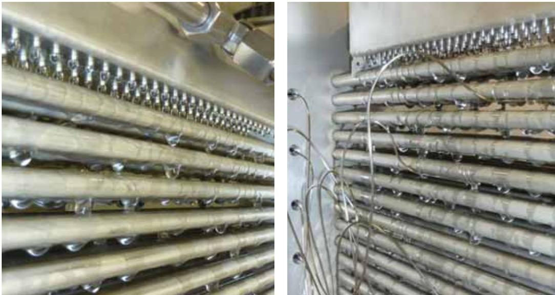
**Fig. 8:** Side view of the falling film on the A/D tube bundle heat and mass exchanger (left) and instrumented – temperature sensors - A/D tube bundle (right); impinging mass flow rate: 30 l/h of water.
