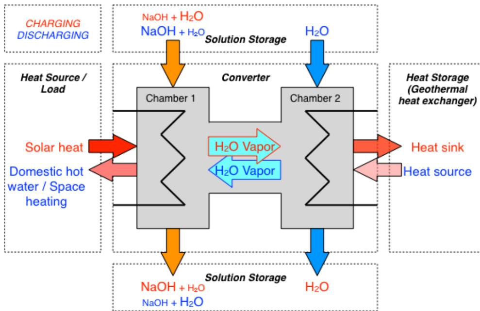
Fig. 1: The concept of the closed sorption heat pump based heat storage (Fumey et al. 2014).
