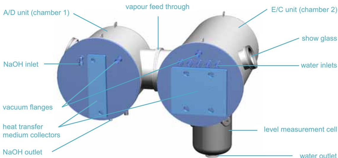
Fig. 2: CAD drawing of the reaction zone with both A/D (left) and E/C unit (right).
