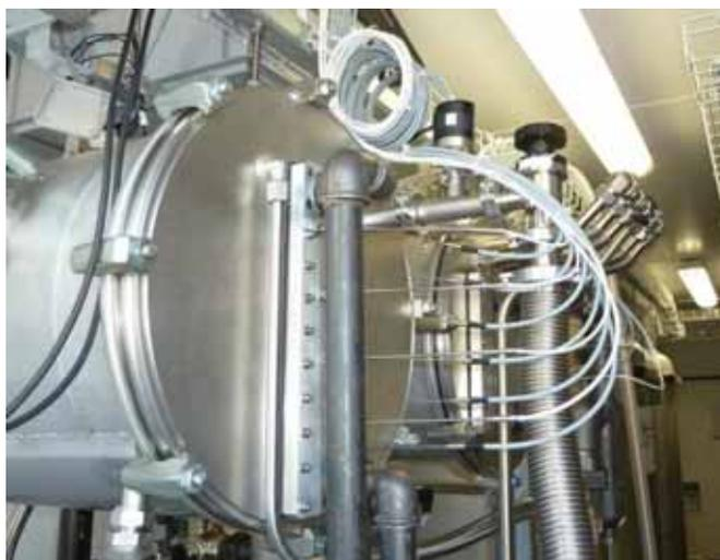
**Fig. 4: View of the installed and measurement sensors equipped reaction zone (A/D unit left, E/C unit right). The vacuum valve - black handle - and the flexible stainless steel vacuum hose - middle right - are used for the ongoing leak test.**
