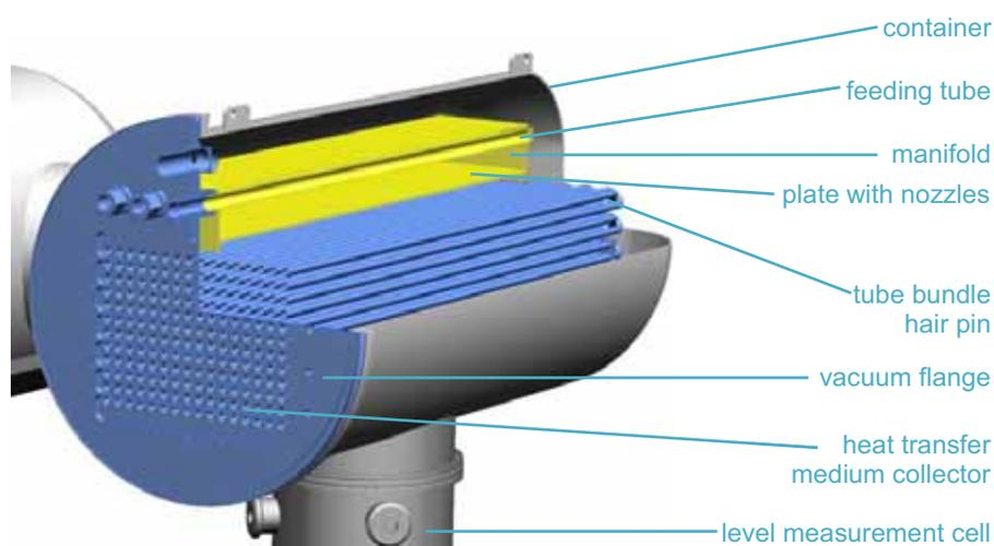
Fig. 3: CAD cross-sectional view of the E/C unit (manifold and tube bundle).
