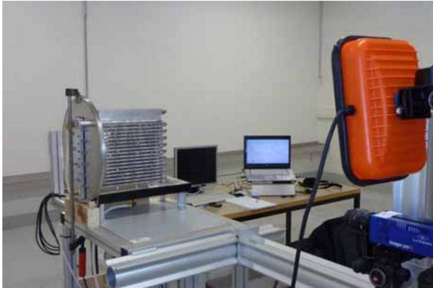
**Fig. 7:** View of the A/D heat and mass heat exchanger during the fluid distribution test.
