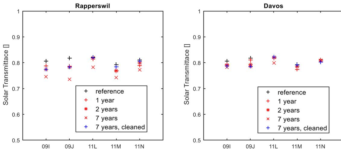
Figure 5: Solar transmittance of all tested AR-coated glass samples after different periods of outdoor exposure in Rapperswil.
