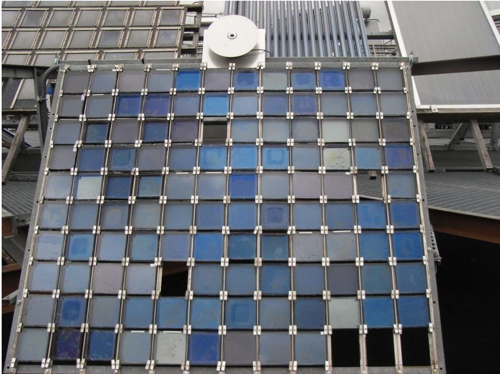
**Figure 1: Outdoor exposure site in Rapperswil with samples mounted on mini collectors.**
