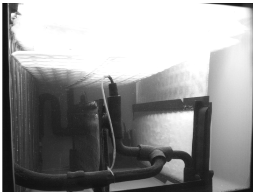
Fig. 2. Side view into the water filled ice storage prototype. Two heat exchangers (centre) during de-icing after several de-icing cycles. The ice plate at the front of the right heat exchanger is still attached to the heat exchanger's surface.
