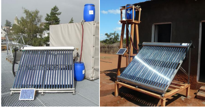
Fig. 7: The left picture shows the overall system installed on the roof at SPF, on the right the system is shown in field-operation in a village in rural Mocambique.
